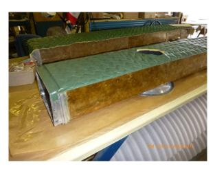
One of the refurbished heater duct sections with a new fabric headliner secured to the top. The sides are covered with mica insulation that was removed, cleaned and reattached after repairs to the metal duct. These will be installed in the main cabin.
