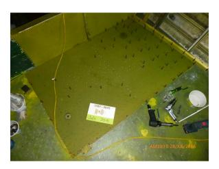
A single new floor panel at the rear of the main cabin required over 1000 rivets. Cleco clips are used to accurately align the panel during riveting.
