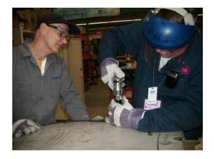
Figure 6: Bill Tate (right) shows new hand Murray Beauliua how to remove old rivets
