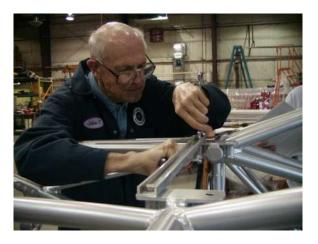
Figure 1: John Corby works on engine mount
