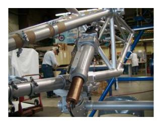
Figure 2: Refurbished engine mount
