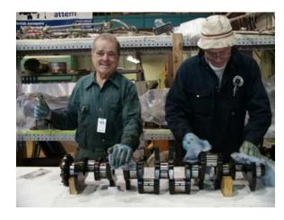
Figure 1: Ted Devey (L), Peter Houston and crankshaft. Oil holes are visible on the crank journals that feed through the connecting rods to the wrist pins on the pistons
