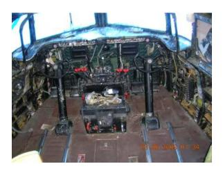
Figure 1: The North Star cockpit stripped of most equipment and fittings, in preparation for repainting
