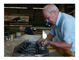
Figure 2: Don Craig working on the oil distribution piping inside the crankcase, rotary stand in the inverted position
