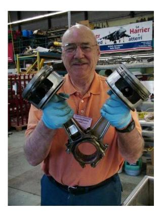
Figure 3: Tim Timmins holding a piston-connecting rod pair that shows the fork-and-blade configuration
