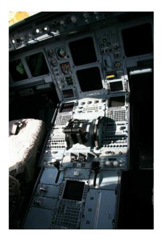
Figure 1: A-330-300 instrument panel
