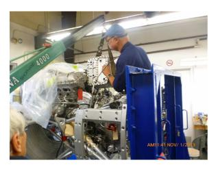
Garry installing the intercooler on engine 3.
