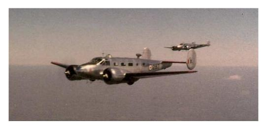
Photo, taken by Tim, of two RCAF C45 Expeditors (military variant of the Beech 18) during the ferry flight he describes in this article. These aircraft were purchased in large numbers during and after WW II for pilot training, navigator training, and as utility transports.
