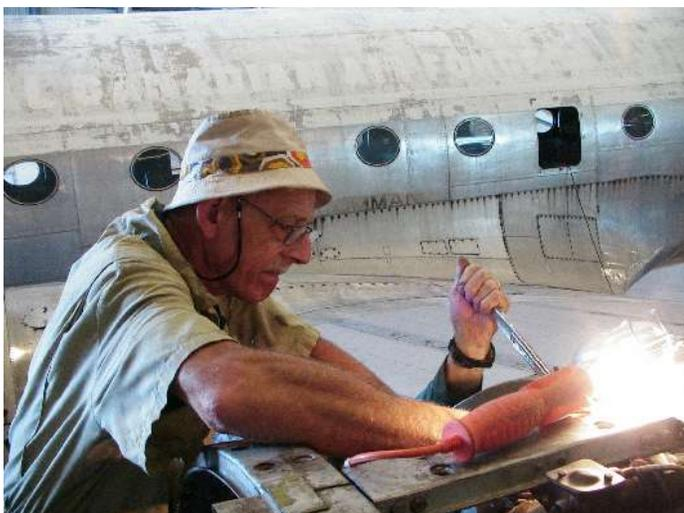
Illustration 1: Tex single-handedly disconnecting port outer engine
