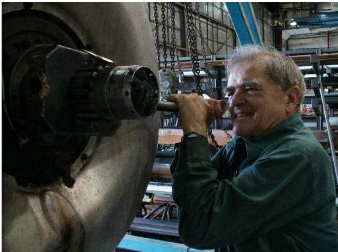
*Illustration 3: Ted "Ironman" Davey checking the compression on engine no.1*
