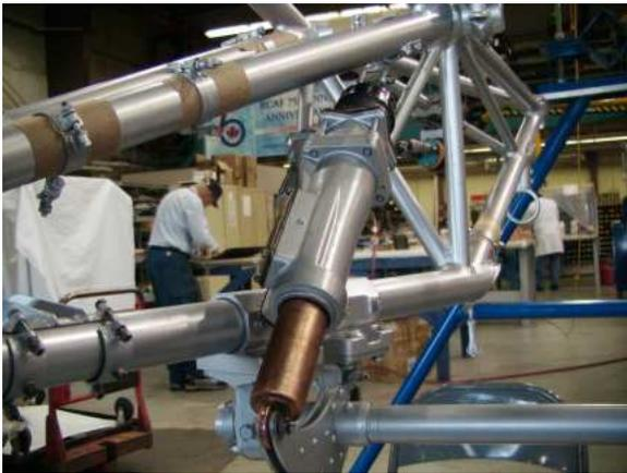
Figure 2: Refurbished engine mount
