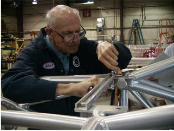
Figure 1: John Corby works on engine mount
