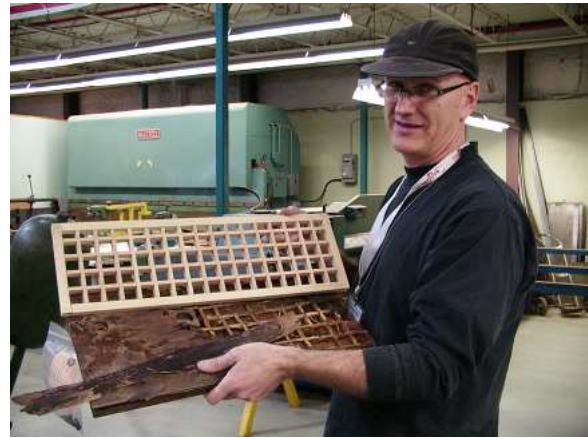
Figure 4.0.2: Murray Beauluia is building replacement sections for the cockpit floor
