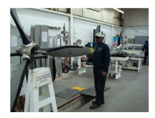
Figure 2: Hope Aero Technician Errol Brown with complete propeller mounted on the balance stand. (Photo courtesy of Hope Aero)
