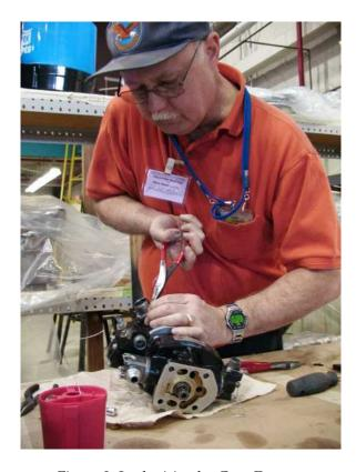
Figure 2: Lockwiring by Gary Dupont
