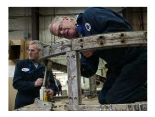
Figure 5: Cowling ring dis-assembly
